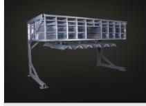
Hardware rack For orderly hardware storage at the sash assembly station
