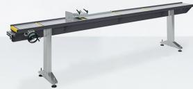
Stop gauge system with profile support, positioning of the stop via handwheel and reading of position on the digital readout. Tolerance on positioning 0.5 mm.
