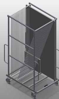
Stable steel construction. Glass sorting. For in-house transportation of sheets of glass. Compartment dividers for 15 sheets of glass. Access is possible from both sides. The glass supporting surface has a rubber profile. Compartment divider with plastic protector. Transport handle on both sides for mobility. Two swivel castors and two fixed rollers.
