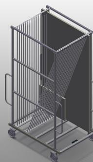
Stable steel construction. Glass sorting. For in-house transportation of sheets of glass. Compartment dividers for 15 sheets of glass. Access is possible from both sides. The glass supporting surface has a rubber profile. Compartment divider with plastic protector. Transport handle on both sides for mobility. Two swivel castors and two fixed rollers.
