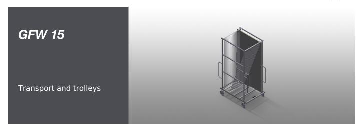
Stable steel construction. Glass sorting. For in-house transportation of sheets of glass. Compartment dividers for 15 sheets of glass. Access is possible from both sides. The glass supporting surface has a rubber profile. Compartment divider with plastic protector. Transport handle on both sides for mobility. Two castors and two fixed rollers.
