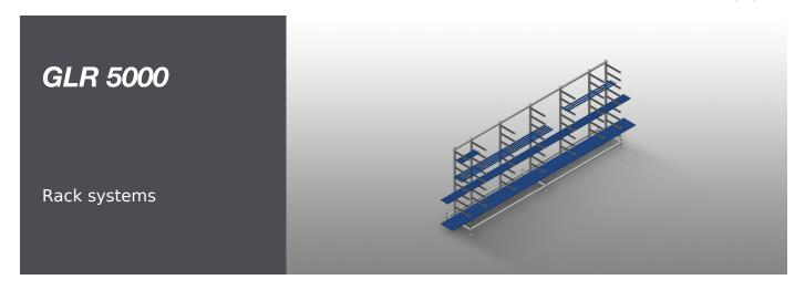
Stable steel construction. Glazing bead rack for horizontal storage of plastic glazing beads. Ideal for storing and sorting glazing beads, e.g. before the glazing bead saw. Seven support arms are evenly spaced along the rack. Four centre supports are adjustable. Nine support arms are freely adjustable, giving variable support arm spacing. Support arms are rubber coated. Well-organised storage provides quick access.
