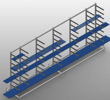
Stable steel construction. Glazing bead rack for horizontal storage of plastic glazing beads. Ideal for storing and sorting glazing beads, e.g. before the glazing bead saw. Seven support arms are evenly spaced along the rack. Four centre supports are adjustable. Nine support arms are freely adjustable, giving variable support arm spacing. Support arms are rubber coated. Well-organised storage provides quick access.
