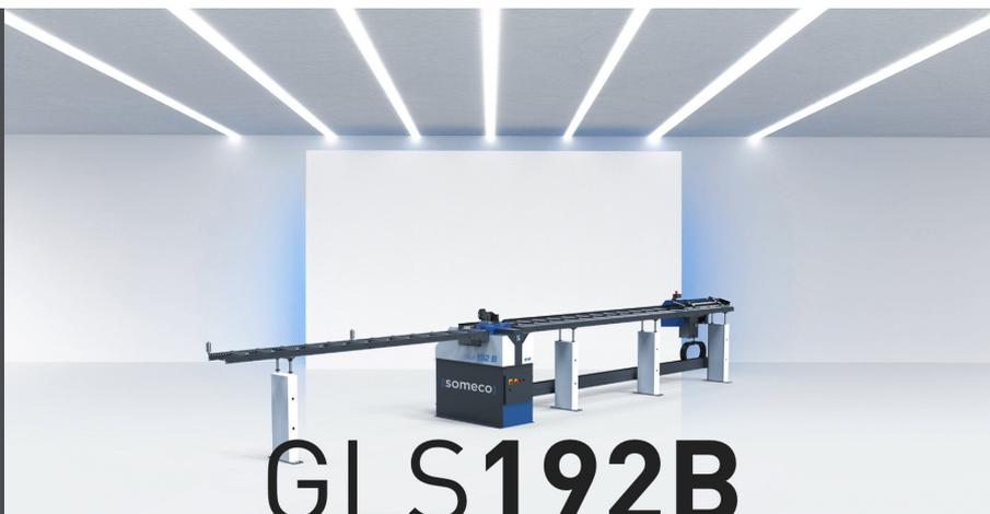
Pneumatic V-cutting saw for 2x45° angle cutting, equipped with special blades arranged one above the other for simultaneous undercutting of the glazing bead web. The machine is equipped as standard with pneumatic, vertical special clamping device which enables the simultaneous processing of glazing beads.
