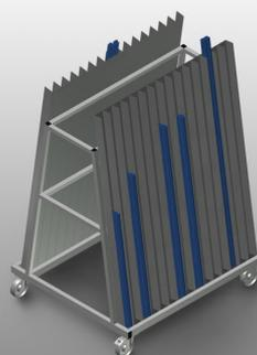
Glazing bead trolley for transportation and sorting of glazing beads. Stable steel construction. Ideal for vertical transportation and sorting of glazing beads. Glazing bead trolley with 30 compartments. 15 compartments per side. Lower supporting surface clad with rubber. Four swivel castors, two of which with locking stop.
