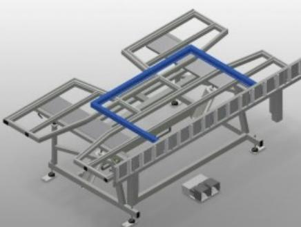
Assembly table for vertical and horizontal assembly. Stable steel construction. Important when switching from vertical to horizontal transportation and vice versa. Ideal for vertical and horizontal assembly. Pneumatic tilting. Table supporting surface with plastic slide bars. Roller support can be lowered pneumatically. 4-fold compressed air supply.
