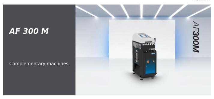
Horizontal end milling machine with manual feed. Milling of intermediate angles,  $+45^{\circ}$  /  $90^{\circ}$  /  $-45^{\circ}$ . Quick cutter change with pneumatic control. Scratch-proof work table. Fully guarded work zone.
