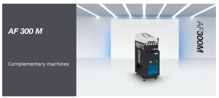
Horizontal end milling machine with manual feed. Milling of intermediate angles, +45° / 90° / -45°. Quick cutter change with pneumatic control. Scratch-proof work table. Fully guarded work zone.
