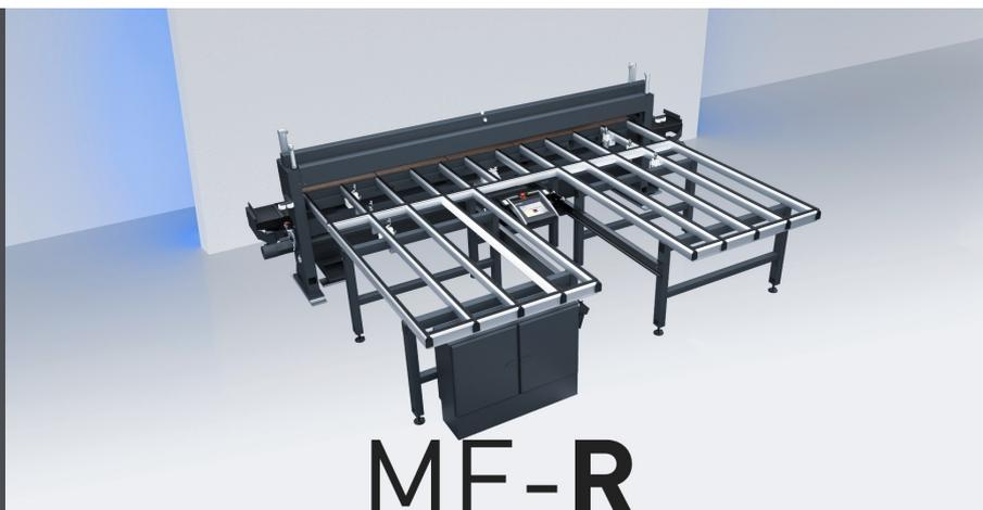
ME-R is a semiautomatic-cycle trimming machine for PVC frames with two controlled axes. It is equipped with a CN cutting unit with adjustable advancement speed.
