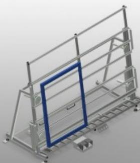
Assembly table for vertical assembly. Stable steel construction. Ideal for vertical assembly. Suitable for lines. Infinitely variable intermediate positions for ergonomic working. Height adjustment by means of pneumatic cylinder. Roller support with steel rollers. Table supporting surface with plastic slide bars. Two horizontally adjustable profile clamps. 4-fold compressed air supply.
