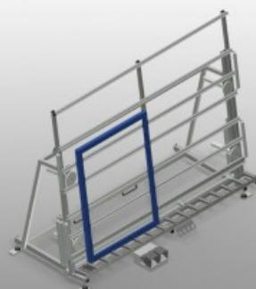
Assembly table for vertical assembly. Stable steel construction. Ideal for vertical assembly. Suitable for lines. Infinitely variable intermediate positions for ergonomic working. Height adjustment by means of pneumatic cylinder. Roller support with steel rollers. Table supporting surface with plastic slide bars. Two horizontally adjustable profile clamps. 4-fold compressed air supply.
