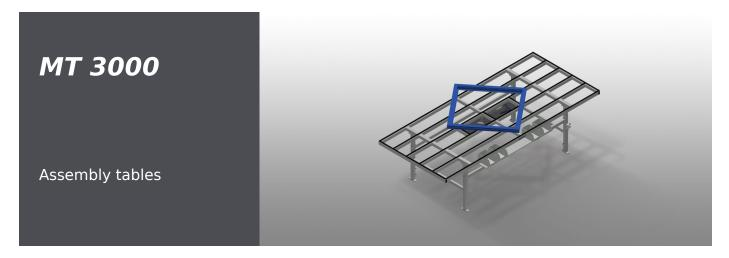
Assembly table for all work tasks on frames and sashes. Stable steel construction. Assembly table for all work tasks on frames and sashes. Table supporting surface with plastic slide bars. Storage tray for setting down tools and accessories. Adjustable height. Practical storage area under the table surface. Four PVC containers for small accessories, hardware and screws. 4-fold compressed air supply. Simple installation with a modular system design.
