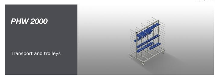
Profile trolley for horizontal storage and transportation of profiles. Stable steel construction. Horizontal profile transportation. Profile trolley with profile supports on both sides. Twelve storage areas per upright. Four castors, two of which have a fixing brake. Options: plastic protector for PHW 1600/2000; number label for PHW 1600/2000.
