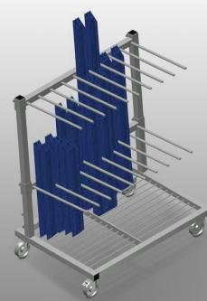
Profile trolley for vertical storage and transportation of profiles. Stable steel construction. Vertical profile transportation. Profile trolley with loading on one side. Easy loading and unloading. Sufficient for 30-40 profile bars. Compartment divider height is adjustable. Supporting surface with bar grid floor. Four swivel castors, two of which with locking stop.
