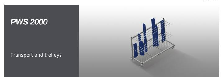
Profile trolley for vertical storage and transportation of profiles. Stable steel construction. Vertical profile transportation. Profile trolley with loading on one side. Easy loading and unloading. Sufficient for 60 – 80 profile bars. Compartment dividers height is adjustable. Supporting surface with bar grid floor. Four swivel castors, two of which with locking stop.
