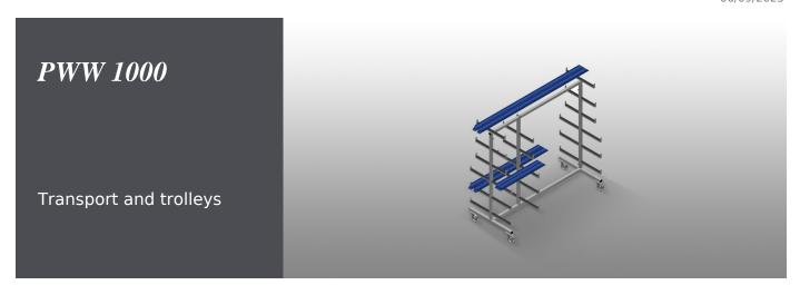
Profile trolley for horizontal storage and transportation of profiles. Stable steel construction. Horizontal profile transportation. Support arms are rubber coated. Profile trolley with profile supports on both sides. Six supports per upright. One centre upright. Four swivel castors, two of which with locking stop.
