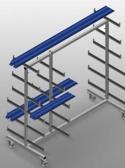
Profile trolley for horizontal storage and transportation of profiles. Stable steel construction. Horizontal profile transportation. Support arms are rubber coated. Profile trolley with profile supports on both sides. Six supports per upright. One centre upright. Four swivel castors, two of which with locking stop.
