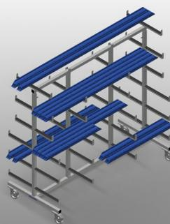
Profile trolley for horizontal storage and transportation of profiles. Stable steel construction. Horizontal profile transportation. Support arms are rubber coated. Profile trolley with profile supports on both sides. Six supports per upright. Two centre uprights. Four swivel castors, two of which with locking stop.
