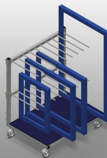
Profile trolley for in-house transportation of frames and sashes. Stable steel construction. Trolley with sorting rack for transportation and storage of frames and sashes. Hardwood supporting surface. Compartment dividers for nine frames. Compartment divider height is adjustable. Four swivel castors, two of which with locking stop.
