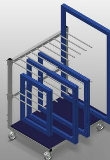
Profile trolley for in-house transportation of frames and sashes. Stable steel construction. Trolley with sorting rack for transportation and storage of frames and sashes. Hardwood supporting surface. Compartment dividers for nine frames. Compartment divider height is adjustable. Four swivel castors, two of which with locking stop.
