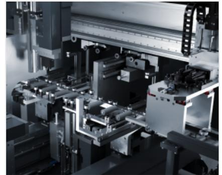
**Milling unit for pvc and steel**
