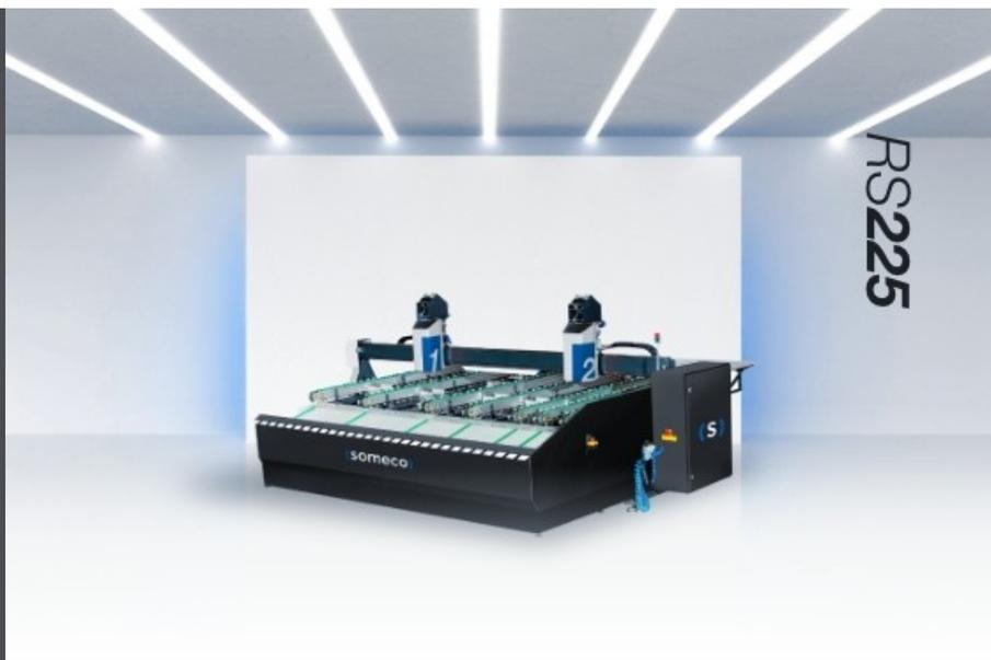
Automatic workbench for the automated screwing. Screwing operation process done simultaneously by two separate fully automatic screwing axis-controlled units. All machine axes are moved by hardened steel ball screw and rack-pinion gear system that provides accuracy and durability. The precision of positioning with 0,1 mm accuracy by high-speed servo on the holder axis. The machine is fully compatible with Processing center in automatic operation.
