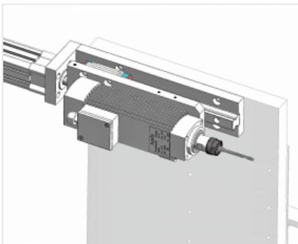
**Drilling unit for wall mounting**
