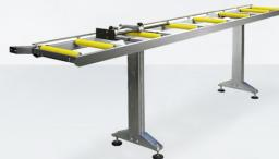
Tubular steel construction with adjustable mounting feet and PVC covered steel rolls. In the version with rolls size 240 mm, roller conveyor length is 3.500 mm.
