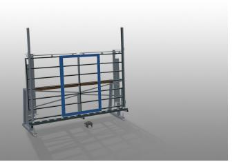
Inspection and glazing unit for glazing and final inspection. Quick and precise assembly of windows, doors and elements. Stable steel construction. Precision ensured through parallel clamping bar pressing technique with manually operated pressing bars. Easy operation by means of foot switch. Pneumatic centring, storage area for tools and 4-fold compressed air supply.
