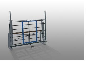
Inspection and glazing unit for glazing and final inspection. Quick and precise assembly of windows, doors and elements. Stable steel construction. Precision ensured through parallel clamping bar pressing technique with manually operated pressing bars. Easy operation by means of foot switch. Pneumatic centring, storage area for tools and 4-fold compressed air supply.
