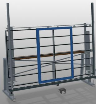
Inspection and glazing unit for glazing and final inspection. Quick and precise assembly of windows, doors and elements. Stable steel construction. Precision ensured through parallel clamping bar pressing technique with manually operated pressing bars. Easy operation by means of foot switch. Pneumatic centring, storage area for tools and 4-fold compressed air supply.
