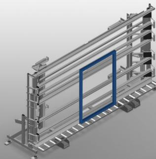
Inspection and glazing unit for glazing and final inspection in individual and serial assembly line production. Quick and precise assembly of windows, doors and elements. Stable steel construction. Precision ensured through parallel clamping bar pressing technique. Height continuously adjustable. Easy operation by means of foot switch. Two pressing bars which fold down and can be moved pneumatically and 4-fold compressed air supply.
