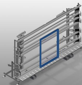
Inspection and glazing unit for glazing and final inspection in individual and serial assembly line production. Quick and precise assembly of windows, doors and elements. Stable steel construction. Precision ensured through parallel clamping bar pressing technique. Height continuously adjustable. Easy operation by means of foot switch. Two pressing bars which fold down and can be moved pneumatically and 4-fold compressed air supply.
