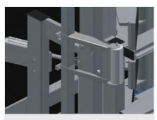
Tilt adjustment of  $0^{\circ}$  -  $8^{\circ}$  (Optional)
