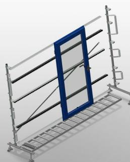
Vertical roller conveyor for transportation and storage of window elements. Stable steel construction. Expandable using modular system design. Vertical roller conveyor for smooth transportation and storage of window elements. Easy handling of window elements. Every roller conveyor unit is 3.000 mm long. Roller conveyor divided into three parts. Plastic slide bars top and bottom. Three mini-roller conveyors with rubber rollers, diameter 50 mm. Basic unit without end rack.
