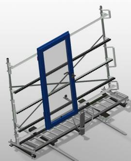
Stable steel construction. Vertical roller conveyor for smooth transportation to the next work task as well as for transportation to storage and sorting of the finished windows. Easy handling of window elements. Every roller conveyor unit is 3.000 mm long. Plastic slide bars top and bottom. Three mini-roller conveyors with rubber rollers, diameter 50 mm. Basic unit with end rack. Vertical roller conveyor on rails with flanged rollers, mobile. Roller conveyor can be rotated 360°.
