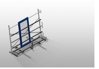
Stable steel construction. Vertical roller conveyor for smooth transportation to the next work task as well as for transportation to storage and sorting of the finished windows. Easy handling of window elements. Every roller conveyor unit is 3.000 mm long. Plastic slide bars top and bottom. Three mini-roller conveyors with rubber rollers, diameter 50 mm. Basic unit with end rack. Vertical roller conveyor on rails with flanged rollers, mobile. Roller conveyor can be rotated 360°.
