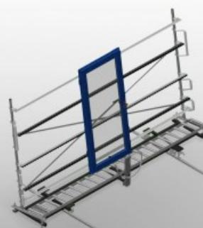
Stable steel construction. Vertical roller conveyor for smooth transportation to the next work task as well as for transportation to storage and sorting of the finished windows. Easy handling of window elements. Every roller conveyor unit is 4.000 mm long. Plastic slide bars top and bottom. Three mini-roller conveyors with rubber rollers, diameter 50 mm. Basic unit with end rack. Vertical roller conveyor on rails with flanged rollers, mobile. Roller conveyor can be rotated 360°.
