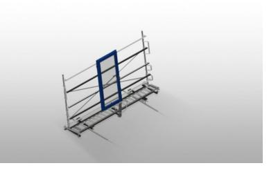
Stable steel construction. Vertical roller conveyor for smooth transportation to the next work task as well as for transportation to storage and sorting of the finished windows. Easy handling of window elements. Every roller conveyor unit is 4.000 mm long. Plastic slide bars top and bottom. Three mini-roller conveyors with rubber rollers, diameter 50 mm. Basic unit with end rack. Vertical roller conveyor on rails with flanged rollers, mobile. Roller conveyor can be rotated 360°.
