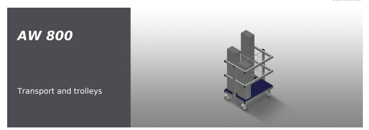
Trolley for transporting and providing a sorted selection of cut-to-length reinforcement profiles. Stable steel construction. Vertical storage and transportation of steel profiles. Compact outside dimensions. Well-organised arrangement of fixed-length profiles. Four swivel castors, two of which with locking stop.
