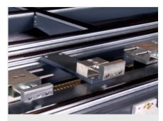
Stop block (Optional) Stop blocks for additional sash widths
