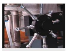
8-fold height adjustment (Optional) 8-fold height adjustment for different screw driving heights
