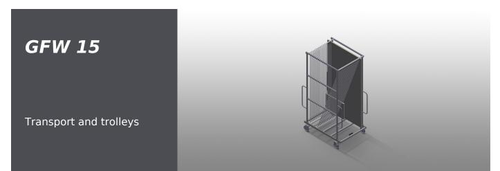
Stable steel construction. Glass sorting. For in-house transportation of sheets of glass. Compartment dividers for 15 sheets of glass. Access is possible from both sides. The glass supporting surface has a rubber profile. Compartment divider with plastic protector. Transport handle on both sides for mobility. Two swivel castors and two fixed rollers.
