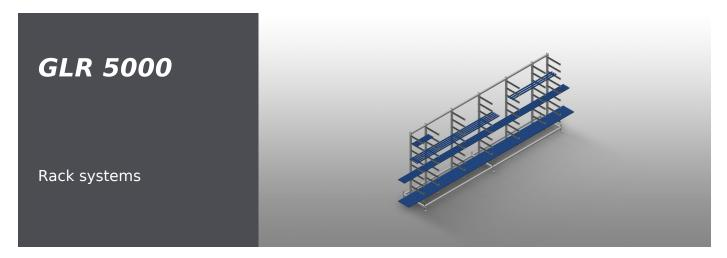
Stable steel construction. Glazing bead rack for horizontal storage of plastic glazing beads. Ideal for storing and sorting glazing beads, e.g. before the glazing bead saw. Seven support arms are evenly spaced along the rack. Four centre supports are adjustable. Nine support arms are freely adjustable, giving variable support arm spacing. Support arms are rubber coated. Well-organised storage provides quick access.
