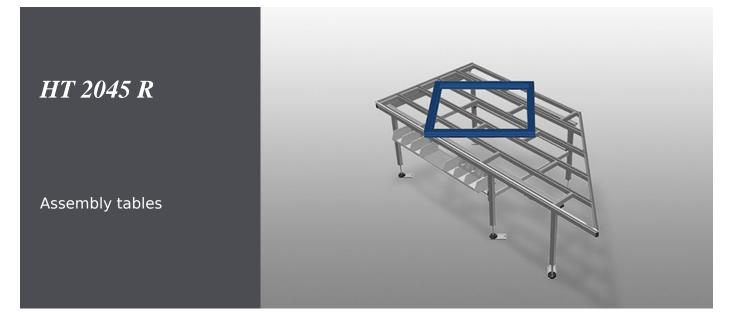
Horizontal table for all work tasks on frames and sashes. Stable steel construction. Angled work table; can be used as a pass-through in the production line or as a buffer zone. Assembly table for all work tasks on frames and sashes. Table supporting surface with plastic slide bars. Storage tray for setting down tools and accessories. Adjustable height. Simple installation with a modular system design.
