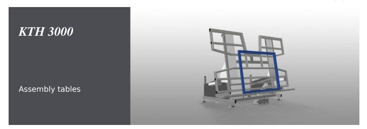
Assembly table for vertical and horizontal assembly. Stable steel construction. Important when switching from vertical to horizontal transportation and vice versa. Ideal for vertical and horizontal assembly. Infinitely variable intermediate positions for ergonomic working. Pneumatic tilting. Pneumatic vertical height adjustment. Table supporting surface with plastic slide bars. Roller support can be lowered pneumatically. Two lateral pneumatic clamps, (lowerable). 4-fold compressed air supply.
