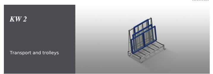
Commissioning trolley for in-house and truck transportation of window elements. Stable steel construction. Trolley for in-house and external transportation. Openings for forklift transportation. Four hooks for crane transportation. Four lashing strap attachment points. Profile supports with rubber surface. Castors can be removed for increased stability of the commissioning trolley in a lorry. Four swivel castors, two of which with locking stop.
