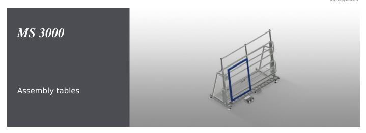
Assembly table for vertical assembly. Stable steel construction. Ideal for vertical assembly. Suitable for lines. Infinitely variable intermediate positions for ergonomic working. Height adjustment by means of pneumatic cylinder. Roller support with steel rollers. Table supporting surface with plastic slide bars. Two horizontally adjustable profile clamps. 4-fold compressed air supply.
