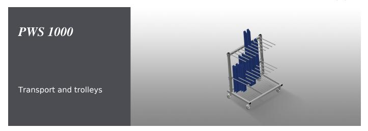
Profile trolley for vertical storage and transportation of profiles. Stable steel construction. Vertical profile transportation. Profile trolley with loading on one side. Easy loading and unloading. Sufficient for 30-40 profile bars. Compartment divider height is adjustable. Supporting surface with bar grid floor. Four swivel castors, two of which with locking stop.
