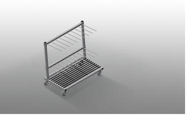
Profile trolley for vertical storage and transportation of aluminium profiles. Stable steel construction. Ideal for transportation and space-saving intermediate storage of cut-to-length profiles. Vertical profile transportation. Sufficient for 30 – 40 profile bars. Compartment divider height is adjustable. Lower supporting surface with rubber strips. Compartment dividers with protective tubing. Rear back support with rubber strips. Four swivel castors, two of which with locking stop.
