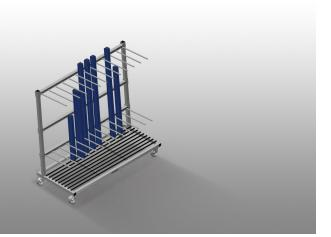
Profile trolley for vertical storage and transportation of aluminium profiles. Stable steel construction. Ideal for transportation and space-saving intermediate storage of cut-to-length profiles. Vertical profile transportation. Sufficient for 12 – 60 profile bars. Compartment divider height is adjustable. Lower supporting surface with rubber strips. Compartment dividers with protective tubing. Rear back support with rubber strips. Four swivel castors, two of which with locking stop.
