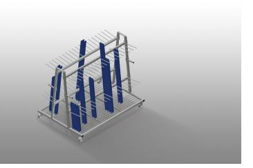
Profile trolley for vertical storage and transportation of profiles. Stable steel construction. Vertical profile transportation. Profile trolley can be loaded on both sides. 18 compartments per side. Easy loading and unloading. Sufficient for 120 – 160 profile bars. Compartment dividers height is adjustable. Supporting surface with bar grid floor. Four swivel castors, two of which with locking stop.
