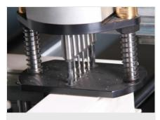
Boring head (Optional) Can be equipped with either 2- or 6spindle boring head
