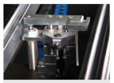
**Rebate stops** Two pneumatically lowerable rebate stops with revolver for up to four
