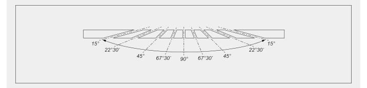
Mechanical adjustment of intermediate angles
