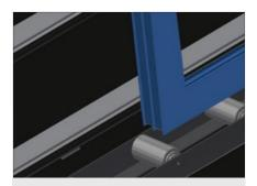
**Roller support** Lower roller conveyor with support roller, L = 120 mm
