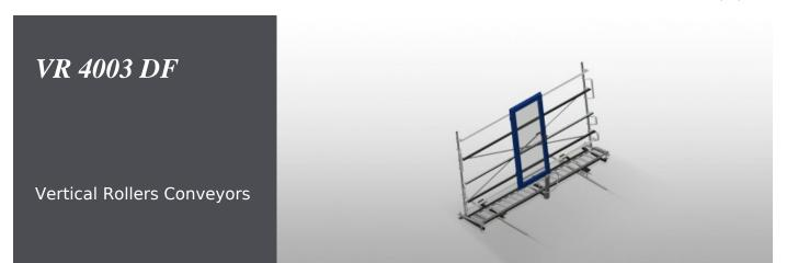
Stable steel construction. Vertical roller conveyor for smooth transportation to the next work task as well as for transportation to storage and sorting of the finished windows. Easy handling of window elements. Every roller conveyor unit is 4.000 mm long. Plastic slide bars top and bottom. Three mini-roller conveyors with rubber rollers, diameter 50 mm. Basic unit with end rack. Vertical roller conveyor on rails with flanged rollers, mobile. Roller conveyor can be rotated 360°.
