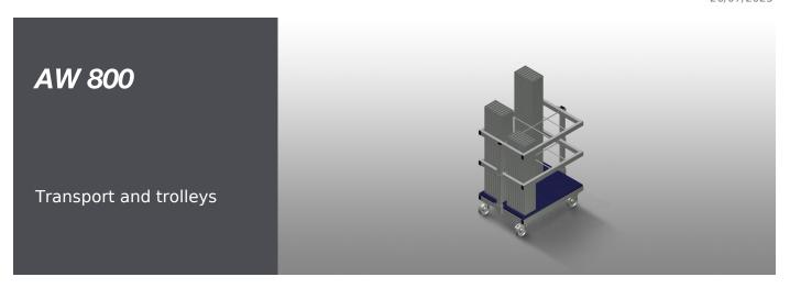
Trolley for transporting and providing a sorted selection of cut-to-length reinforcement profiles. Stable steel construction. Vertical storage and transportation of steel profiles. Compact outside dimensions. Well-organised arrangement of fixed-length profiles. Four swivel castors, two of which with locking stop.
