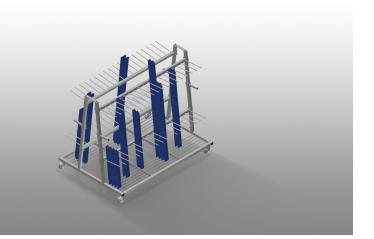
Profile trolley for vertical storage and transportation of profiles. Stable steel construction. Vertical profile transportation. Profile trolley can be loaded on both sides. 18 compartments per side. Easy loading and unloading. Sufficient for 120 – 160 profile bars. Compartment dividers height is adjustable. Supporting surface with bar grid floor. Four castors, two of which have a fixing brake. Option: plastic protector for PWS 4000.
