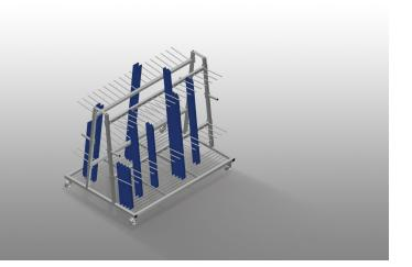
Profile trolley for vertical storage and transportation of profiles. Stable steel construction. Vertical profile transportation. Profile trolley can be loaded on both sides. 18 compartments per side. Easy loading and unloading. Sufficient for 120 – 160 profile bars. Compartment dividers height is adjustable. Supporting surface with bar grid floor. Four swivel castors, two of which with locking stop.
