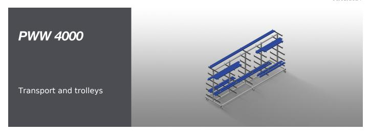
Profile trolley for horizontal storage and transportation of profiles. Stable steel construction. Horizontal profile transportation. Easy transportation of profile raw materials and cut-to-size profiles. Support arms are rubber coated. Profile trolley with profile supports on both sides. Six supports per upright. Three centre uprights. Six castors, two of which have a fixing brake. Option: individual centre upright.
